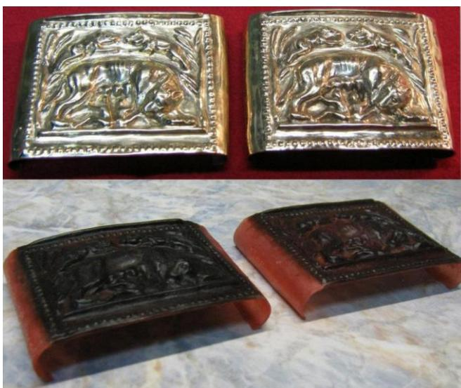
After many experiments I finally managed to find a way to produce bracket on a ancient way by pulling, distortion and hammering! Ears bending was the hardest thing .So with the new technology I've done ancient original thickness of 0.5 mm and excellent quality.
