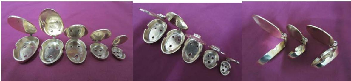
The hinge is mounted monolithically only in one part on the lid. The other should be tightened by knocking around the axis. This complicates the production of wax models.
